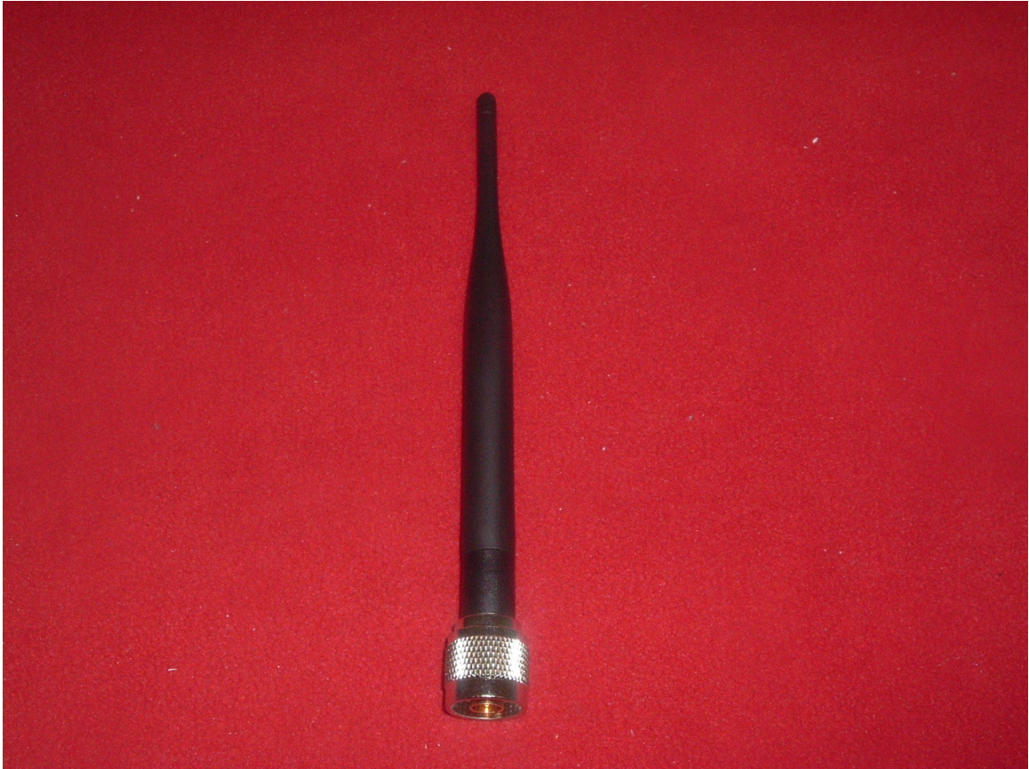
Figure 1: Antenna 1 Omni Antenna 5.5 dBi Gain
