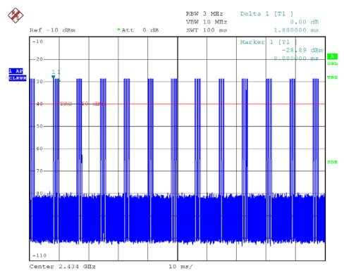
Timing Plot – Pursuant to FCC Part 15 Section 15. 249 Requirement
