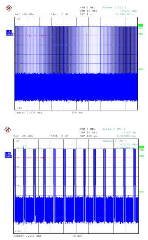
Timing Plot – Pursuant to FCC Part 15 Section 15. 249 Requirement
