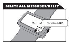
Turning band **OFF** deletes all messages. Turn Band over and SWITCH it **OFF**. Band will RESET when turned back ON. Module resets by turning off and on.
