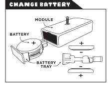
REMOVE MODULE from Band. LOOSEN center screw.
