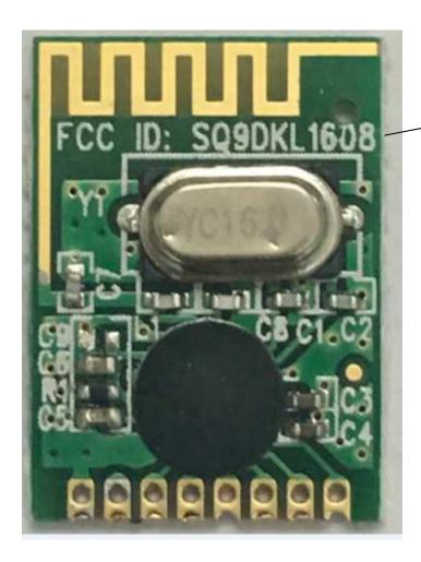
The FCC ID Label is to be silkscreen printed on the Front of Module PCB
