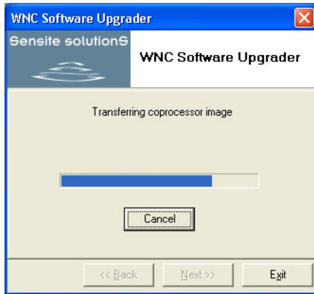
Wait until the transfer is completed. After software upgrade for both processors has finished successfully, both software images are in the WNCs internal volatile memory. Do not power cycle the WNC!
