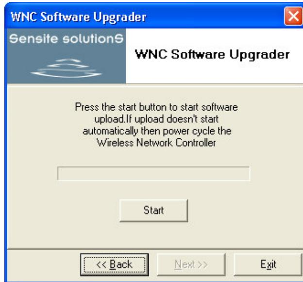
6. Click "Start". Depending on the existing software versions in the WNC the upload will start automatically, or the WNC needs to be power-cycled.
