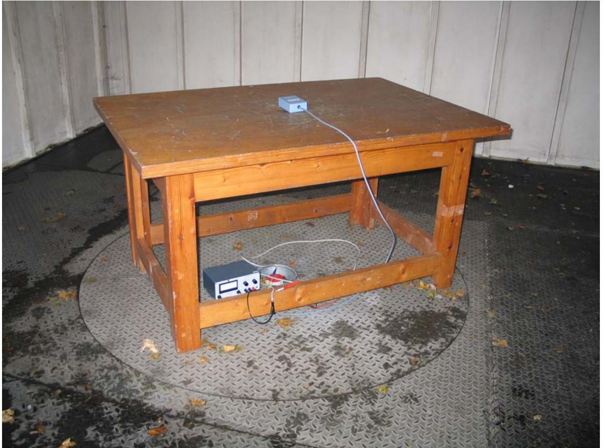
Photograph 3: Table of Open Area Test Site
