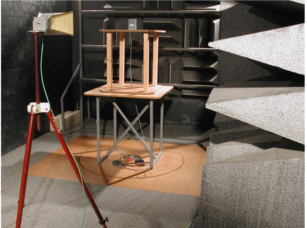
Photograph 1: Test setup in Anechoic Chamber
