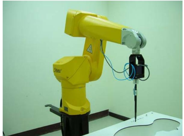
Fig. 5.2 Probe setup on robot
