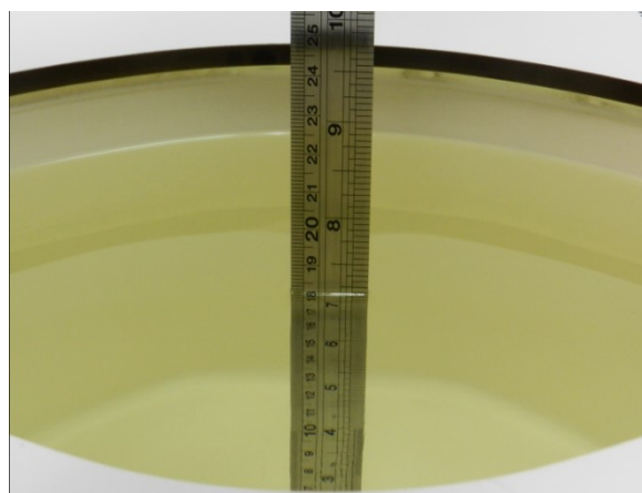
Fig 11.2 Photo of Liquid Height for Body SAR
