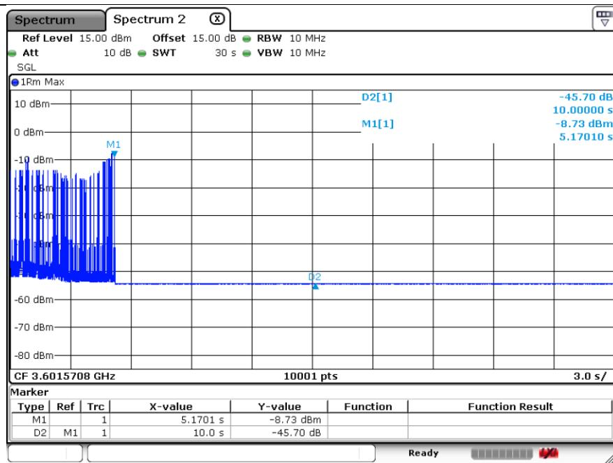
[Step 5] Configure SAS granted CBSD to operate at frequency 3670-3690MHz & power level 8dBm/MHz
