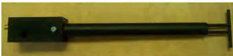
Figure 1 – MVG COMOSAR Validation Dipole
