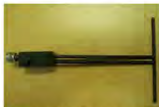
Figure 1 – MVG COMOSAR Validation Dipole
