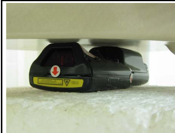
C. The back of the EUT face to the phantom with 0mm-separation distance. (For thick battery)
