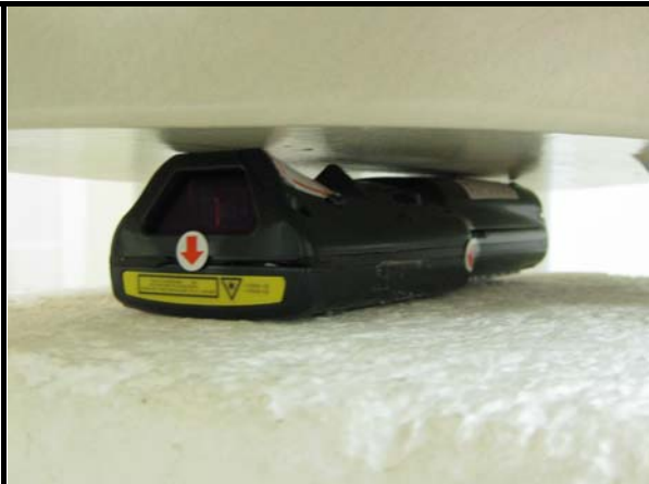
B. The back of the EUT face to the phantom with 0mm-separation distance. (For thin battery)
