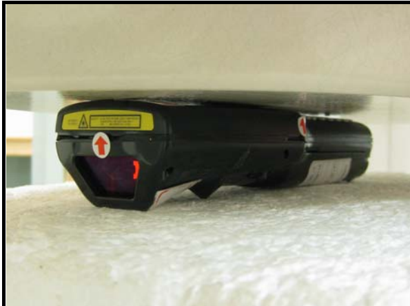
A. The front of the EUT face to the phantom with 0mm-separation distance. (For thin battery)
