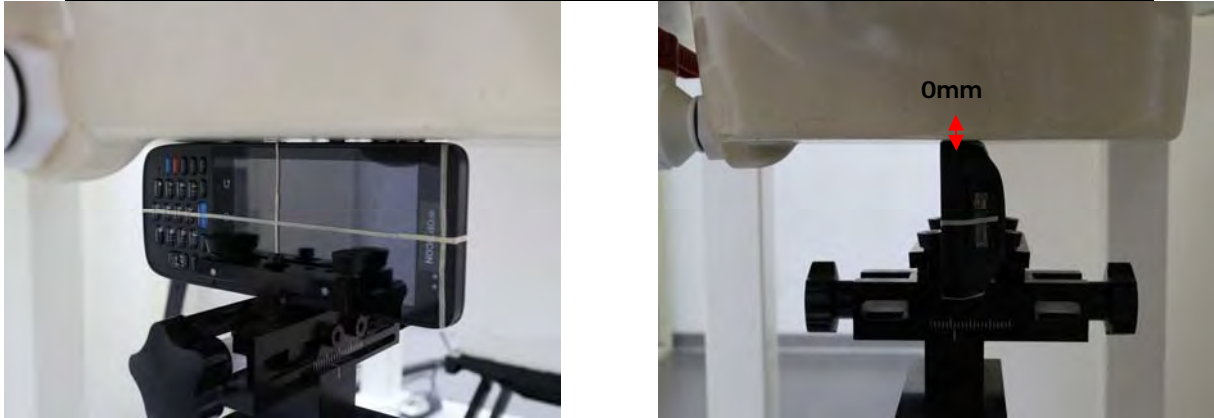
Fig.12 EUT Left side to flat phantom
