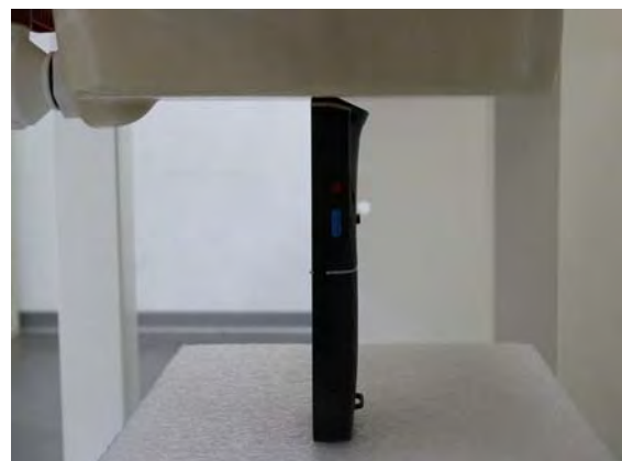
Fig.11 EUT Top side to flat phantom
