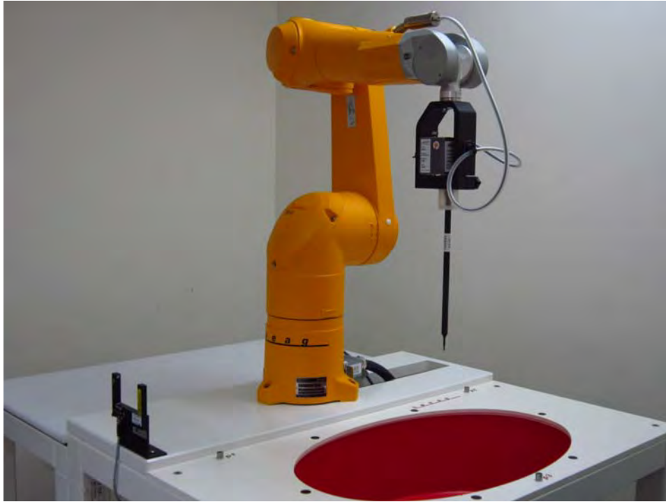
Fig.1 Photograph of the SAR measurement system
