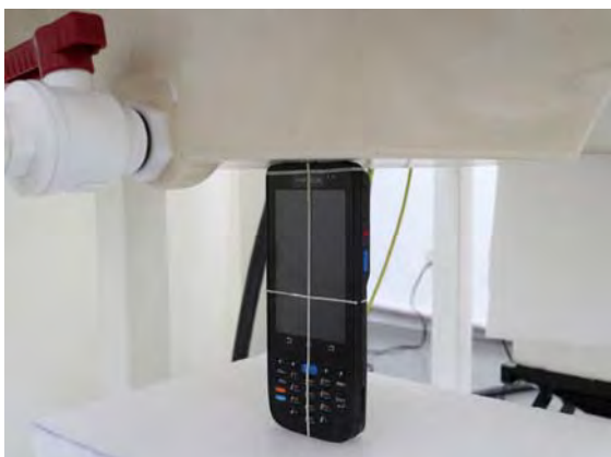
Fig.11 EUT Top side to flat phantom
