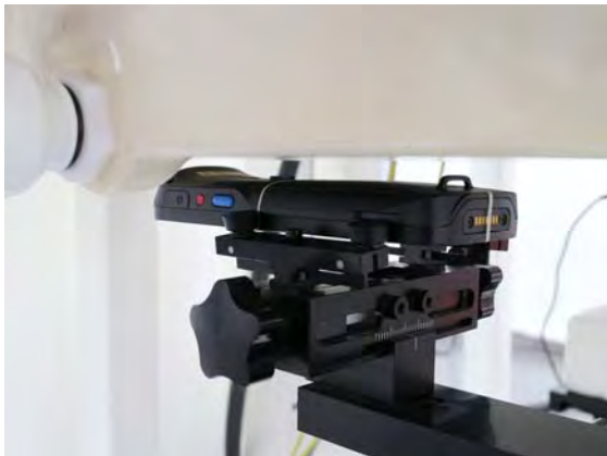
Fig.8 EUT Back side to flat phantom
