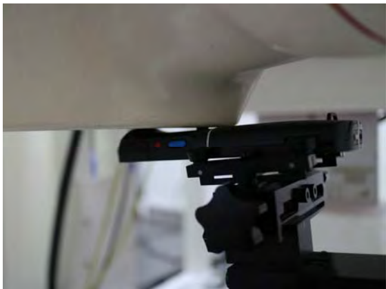
Fig.10 EUT Back side to flat phantom
