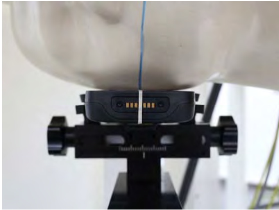
Fig.3 Right Head Section / Cheek-Touch Position
