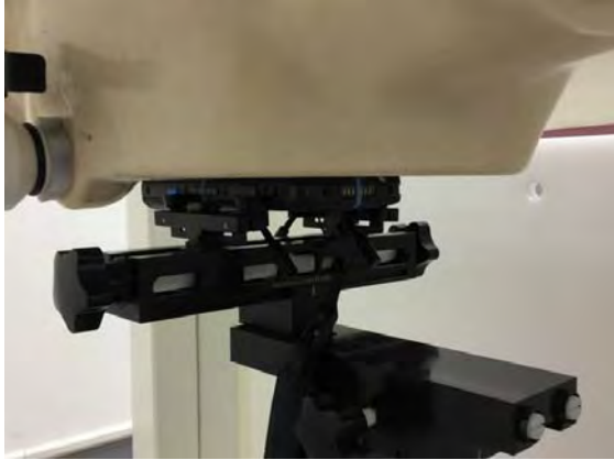
Fig.9 EUT Front side to flat phantom
