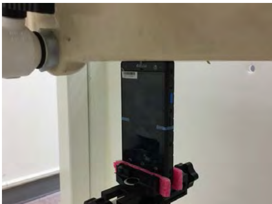
Fig.11 EUT Top side to flat phantom
