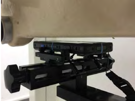
Fig.7 EUT Front side to flat phantom
