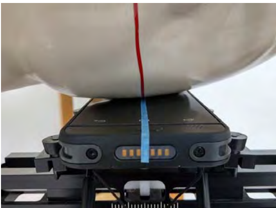
Fig.5 Left Head Section / Cheek-Touch Position
