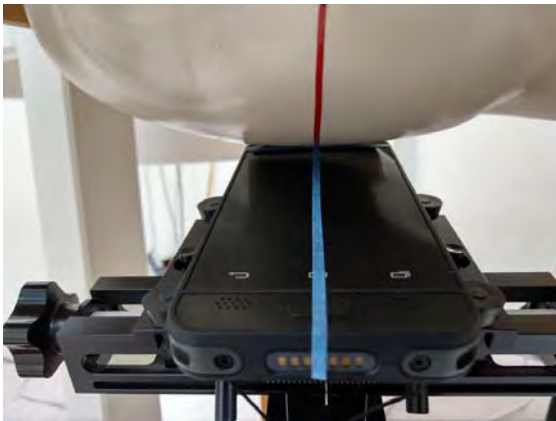
Fig.4 Right Head Section / Ear-Tilt Position(15°)
