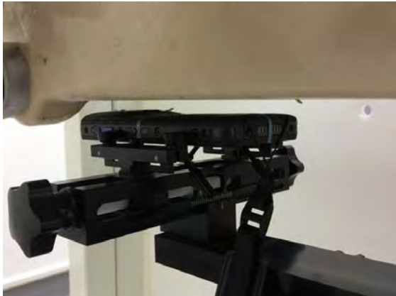
Fig.8 EUT Back side to flat phantom
