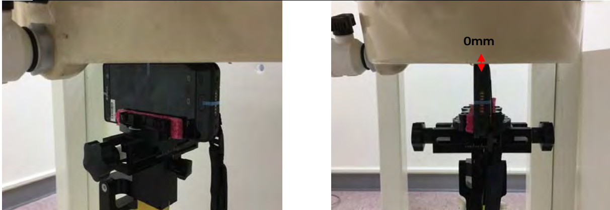
Fig.12 EUT Right side to flat phantom
