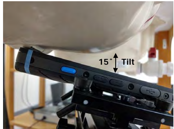
Fig.4 Right Head Section / Ear-Tilt Position(15°)
