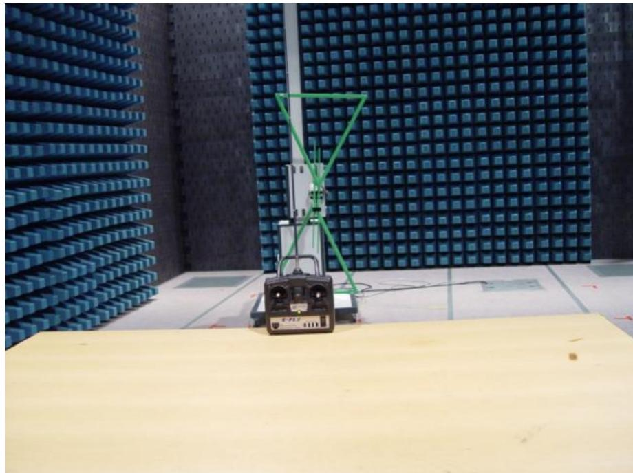
**Test Setup for Radiated Disturbance Test**
