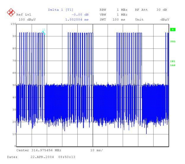
41 pulses @ 1.002 ms each = 41.082 ms ON time. 20 log (41.082 ms / 100 ms) = correction factor of 7.72 dB
