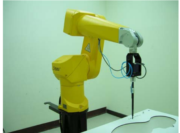
Fig. 5.2 Probe setup on robot
