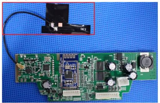
The antenna is integrated on the main PCB and no consideration of replacement. The best case gain of the antenna is 0 dBi.
