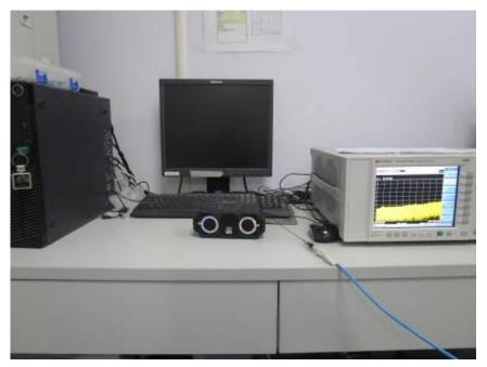
1.2 Conducted Emissions at AC Power Line (150kHz-30MHz) Test Setup
