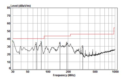
Condition: 3m VERTICAL Job No. : 02963CR Test mode: f
