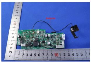
The antenna uses a unique coupling to the intentional radiator and no consideration of replacement. The best case gain of the antenna is 4dBi.
