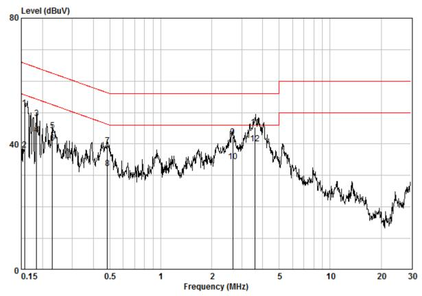
Site : Shielding Room Condition : CE NEUTRAL Job No. : 01463CR Test Mode : TX + Charge
