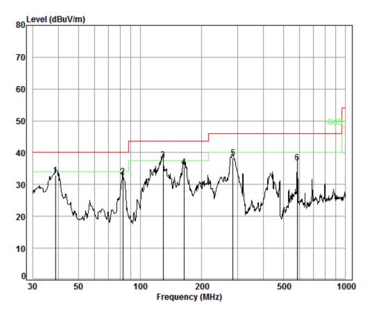
Condition: 3m Vertical Job No. : 01463CR Test mode: TX+Charge
