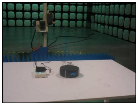
1.2 CONDUCTED EMISSION TEST SETUP
