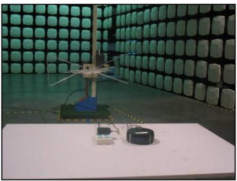
Above 1 GHz: (full anechoic chamber)
