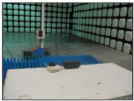
**Conducted Emission Test Setup**
