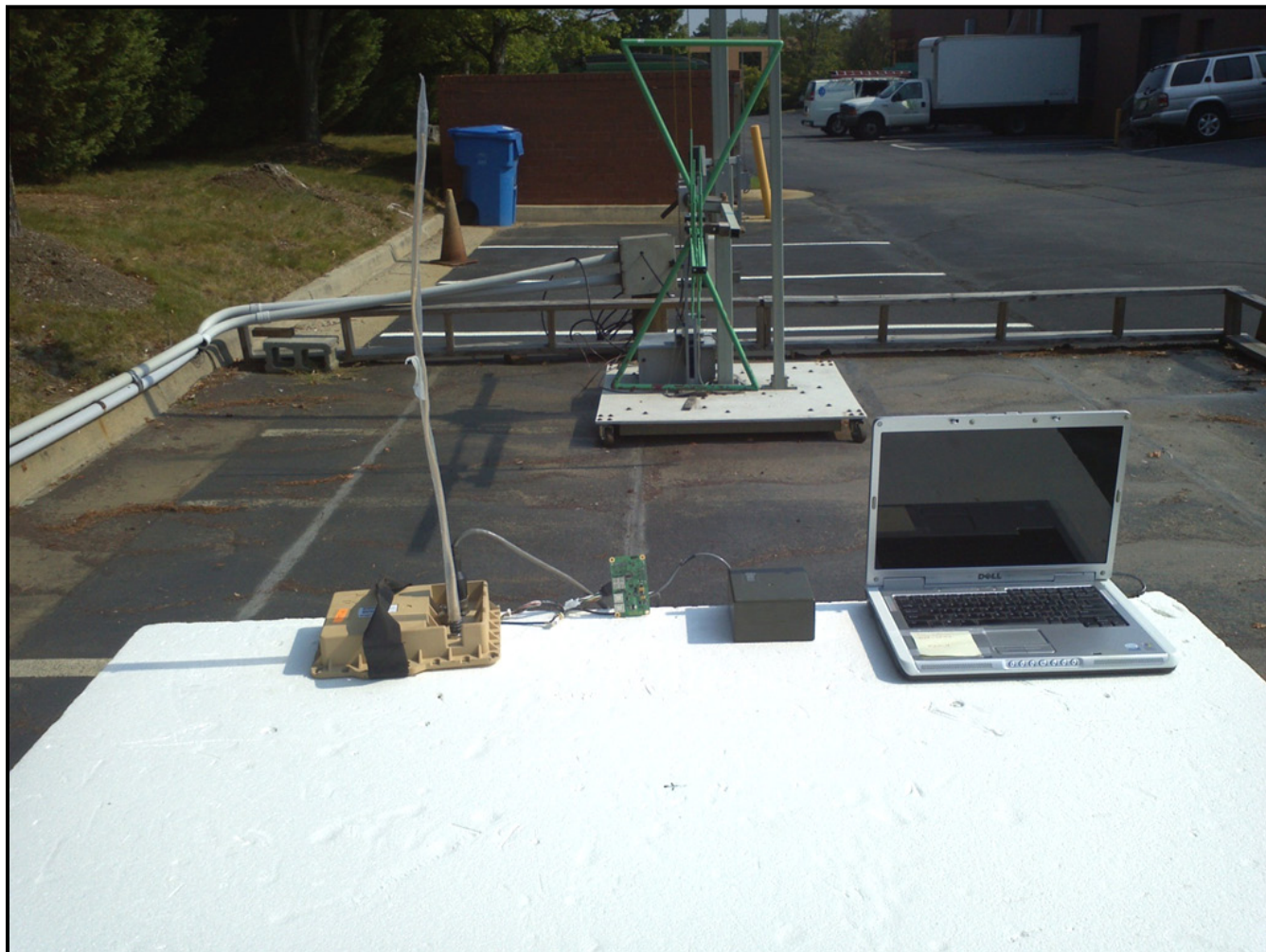
Photograph 1: Radiated Emissions – Front View – Whip Antenna
