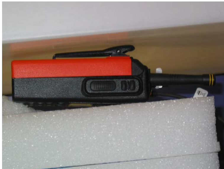
Back Face Test Position 0 mm Gap With Mic
