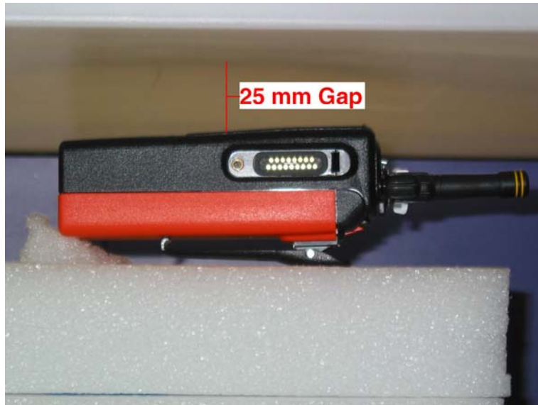
Face Test Position 25 mm Gap
