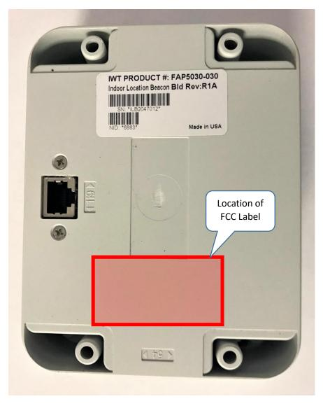
The FCC label will be located on the back of the ILB enclosure. The RED highlighted area shows where the label will be affixed.
