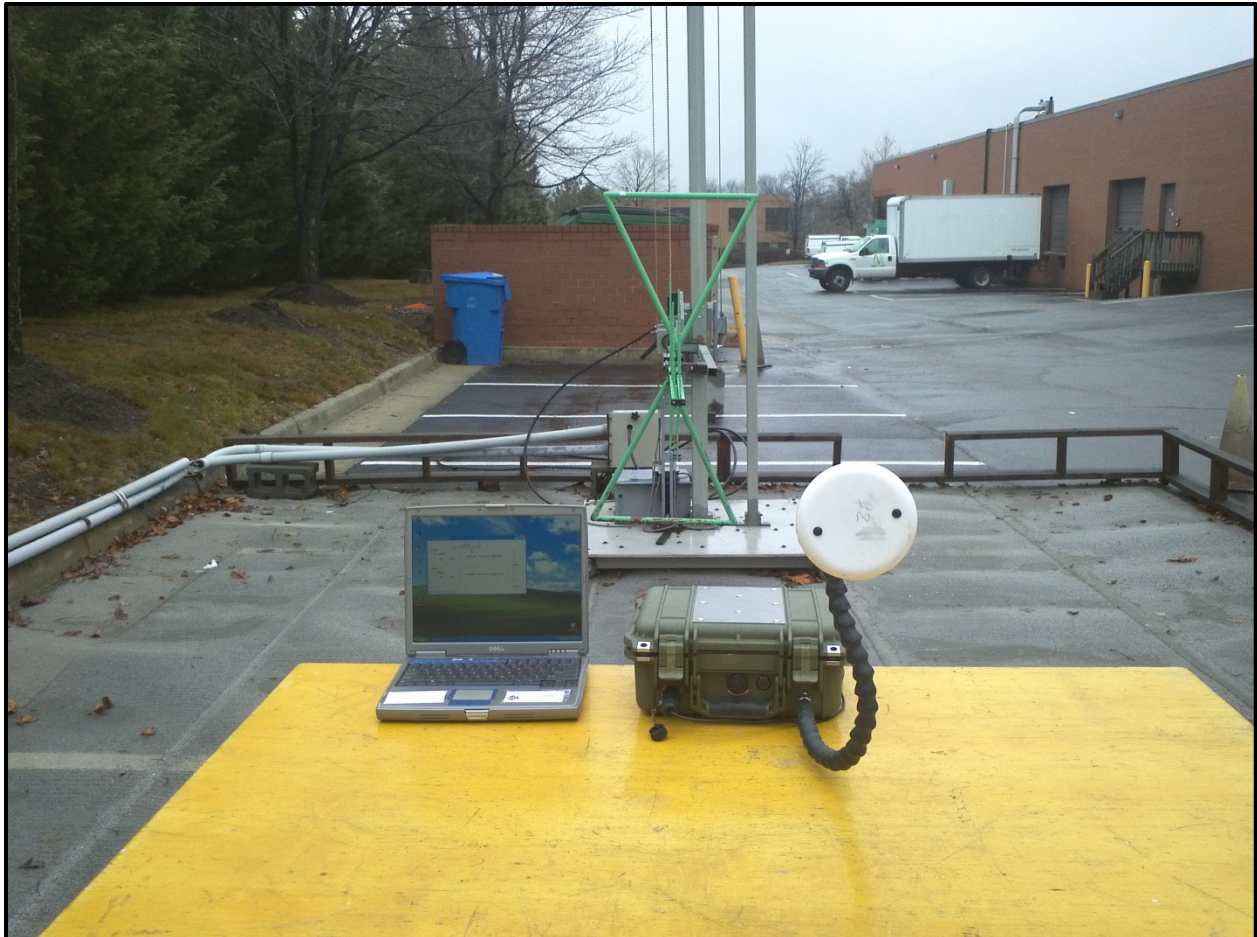
Photograph 1: Radiated Testing – Front View with Omni Antenna
