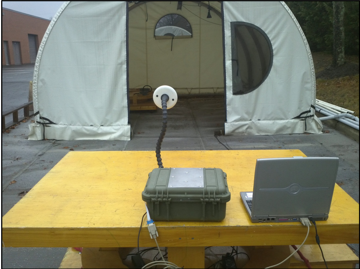
Photograph 2: Radiated Testing – Back View with Omni Antenna
