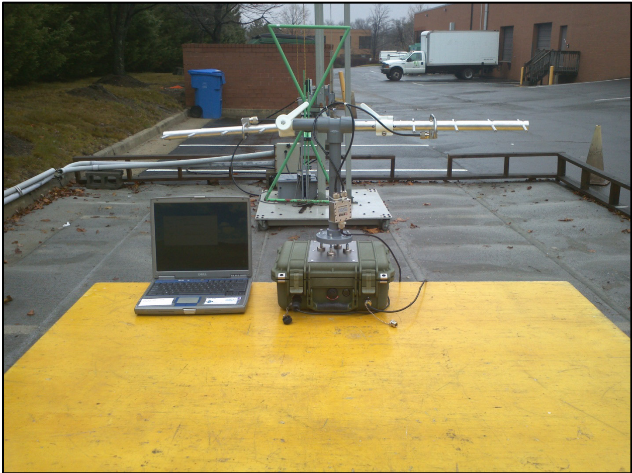
Photograph 3: Radiated Testing – Front View with Yagi Antenna
