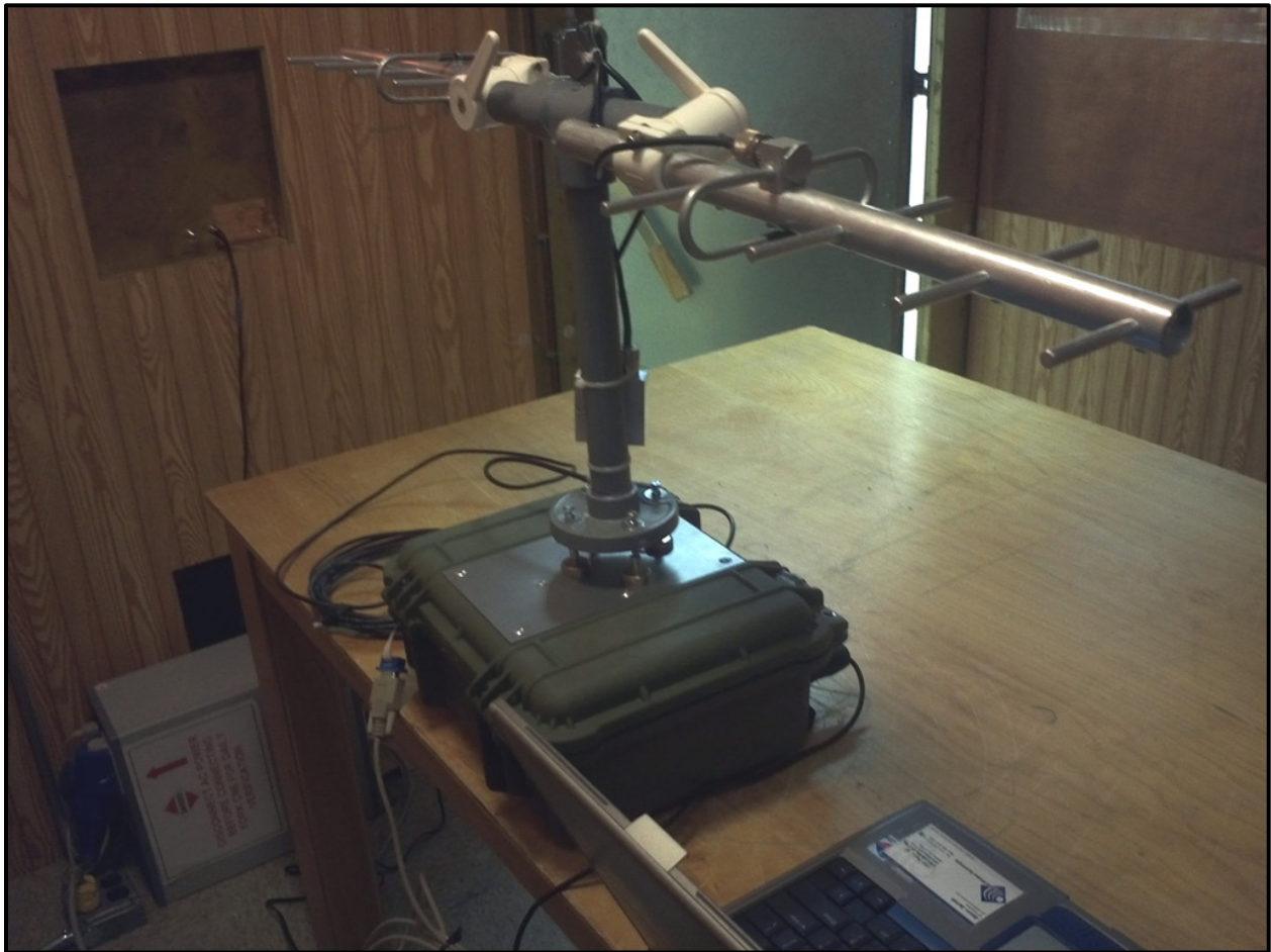
Photograph 8: Conducted AC Testing – Back View with Yagi Antenna
