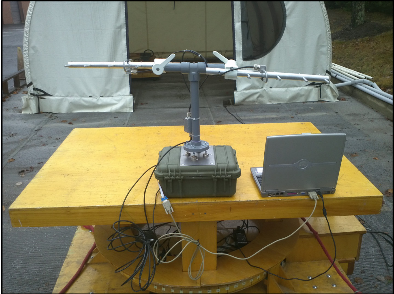
Photograph 4: Radiated Testing – Back View with Yagi Antenna
