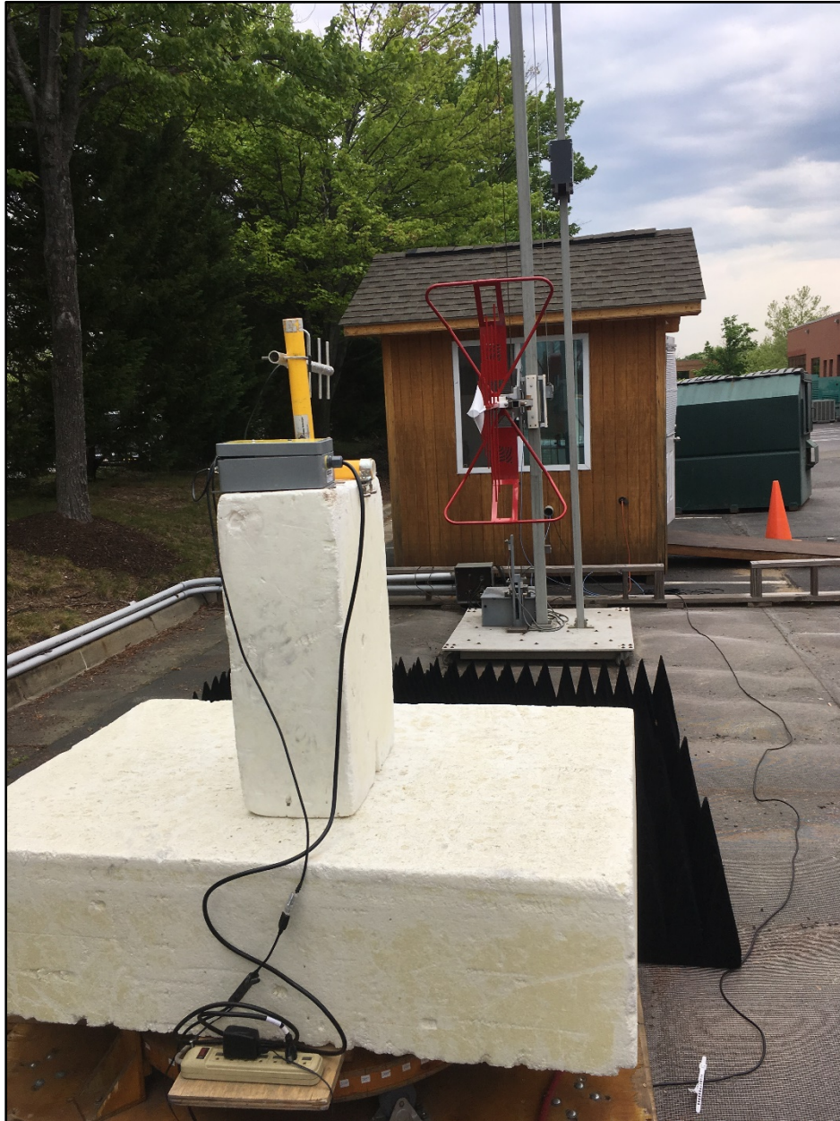
Photograph 8: Yagi Antenna - Back View (Above 1 GHz)
