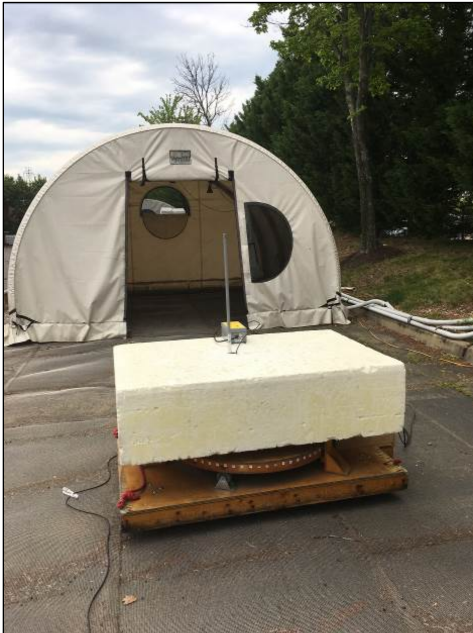
Photograph 1: Omni Antenna - Front View (Below 1 GHz)
