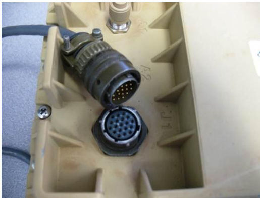
Plug pin end into J1 receptacle on UGS Node (a)
