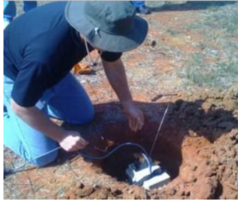
Figure 9 – Coyote UGS node being emplaced in hole
