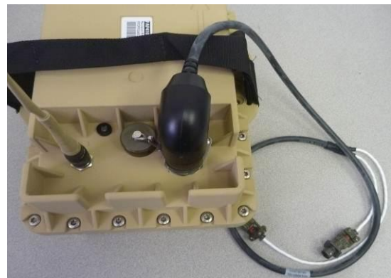
PIR connect to J2 or J3 on MIDs Accessory (b)
