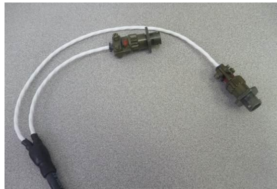
Plug socket end into receptacle on MIDs Accessory
