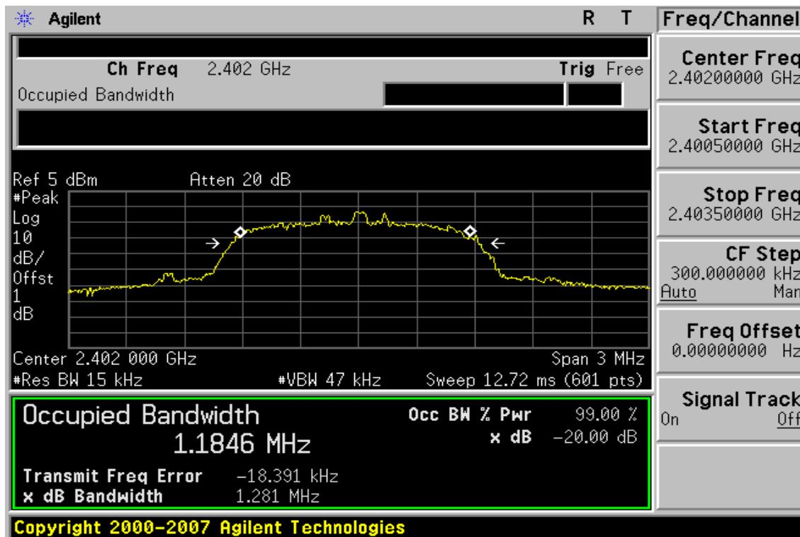
**20dB Bandwidth Test Data CH-Mid**
