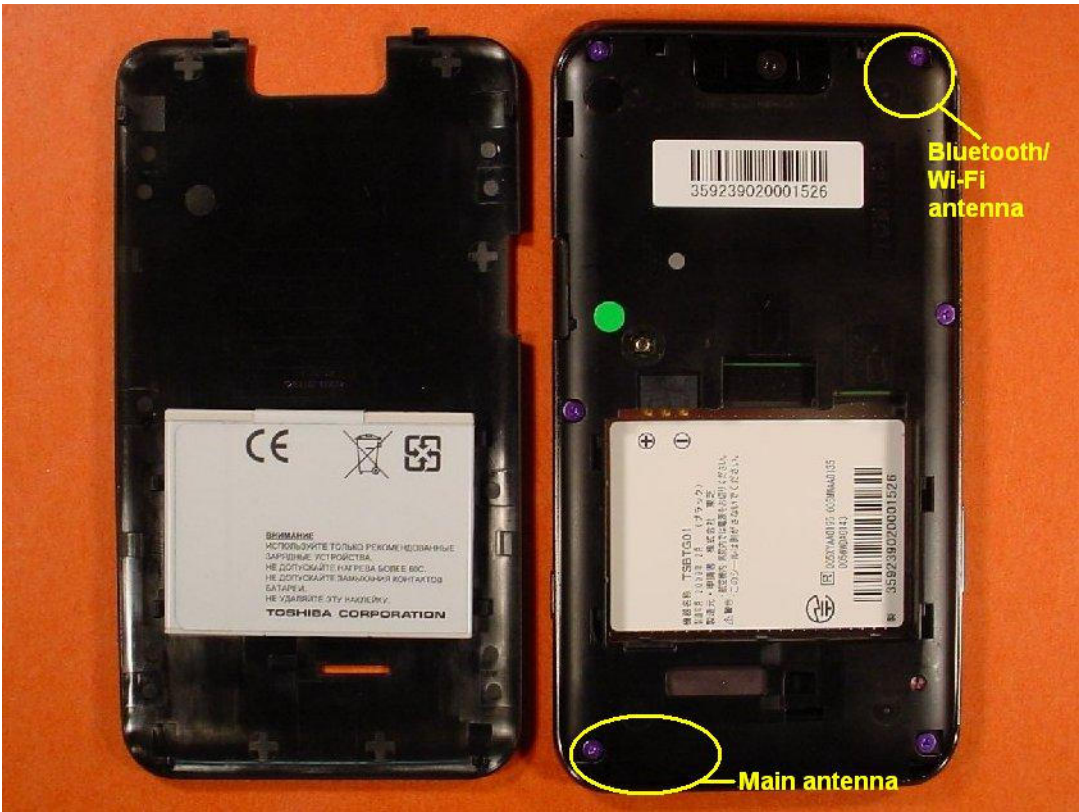
Photo 6: DUT - rear view (open) without battery
