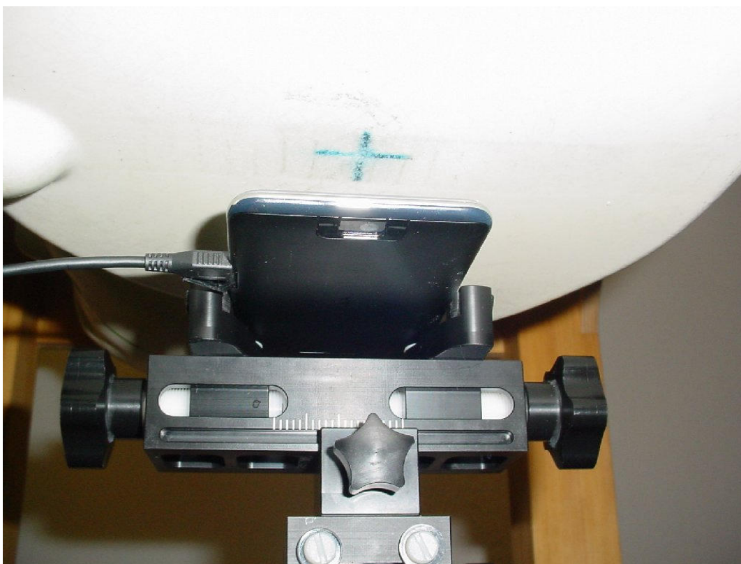
Photo 20: Test position body worn rear side (15 mm distance)
