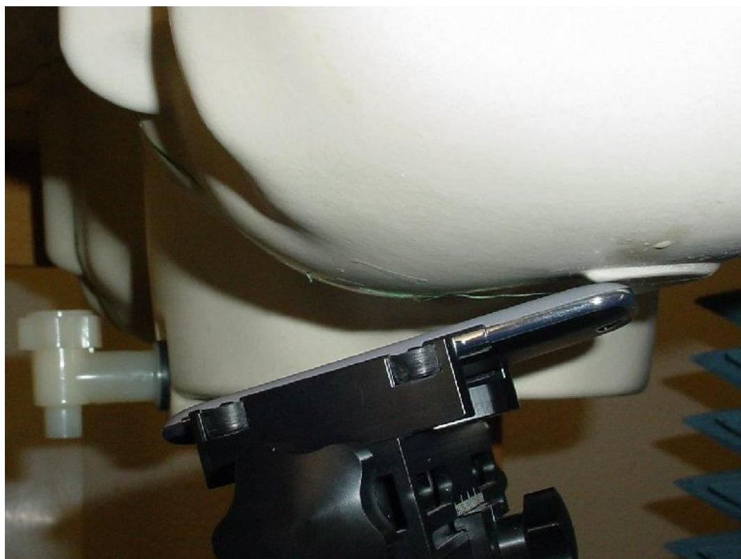
Photo 12: Test position left hand tilted 15°
