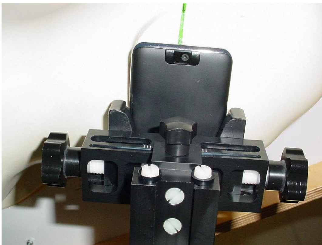
Photo 16: Test position right hand tilted 15°
