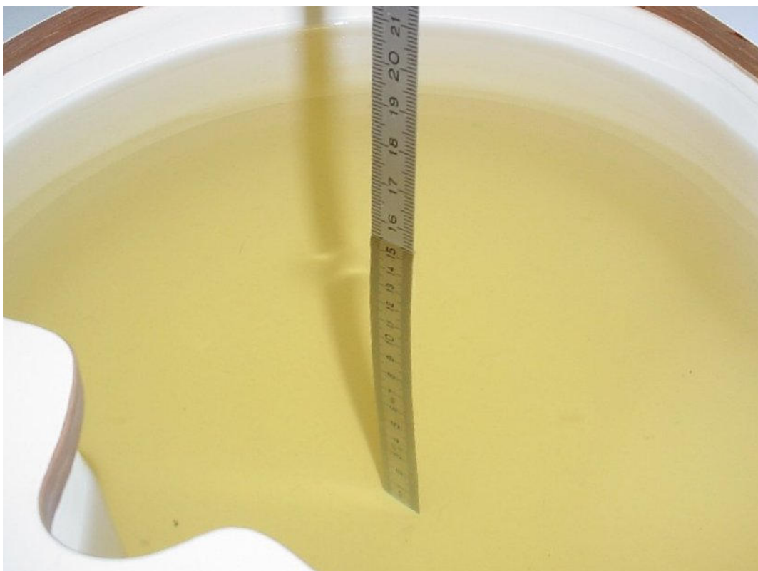
Photo 22: Liquid depth 850 MHz head simulating liquid
