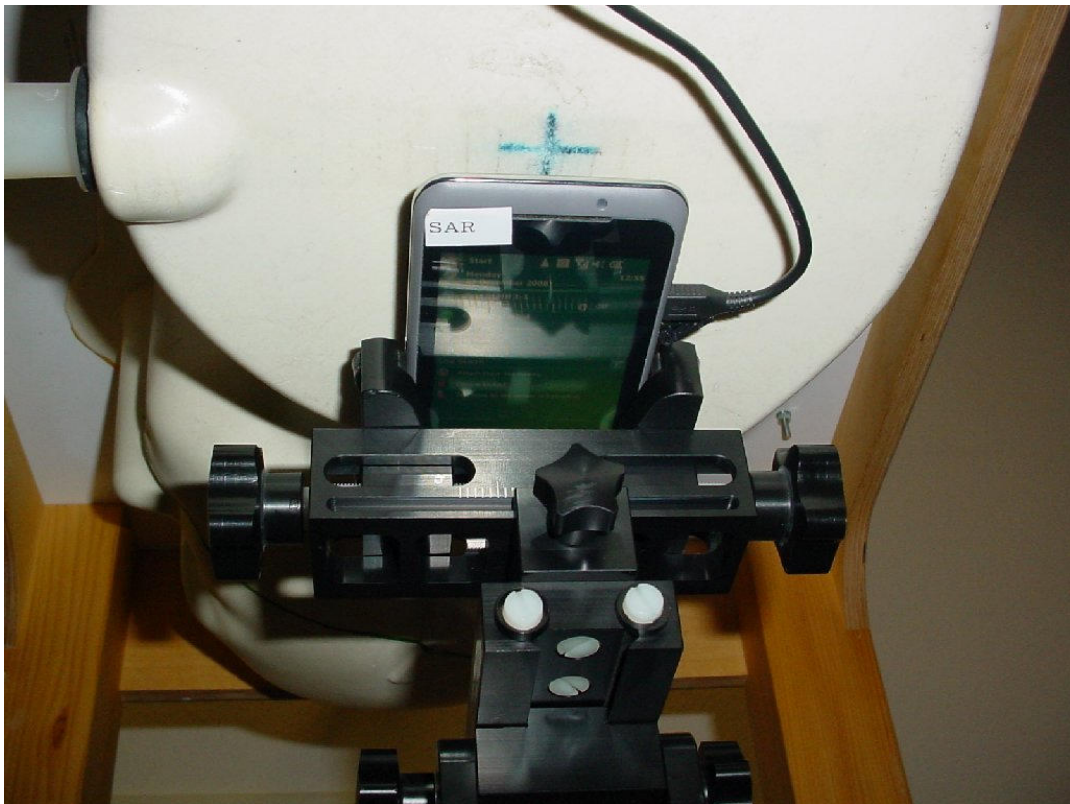
Photo 21: Test position body worn rear side (15 mm distance)
