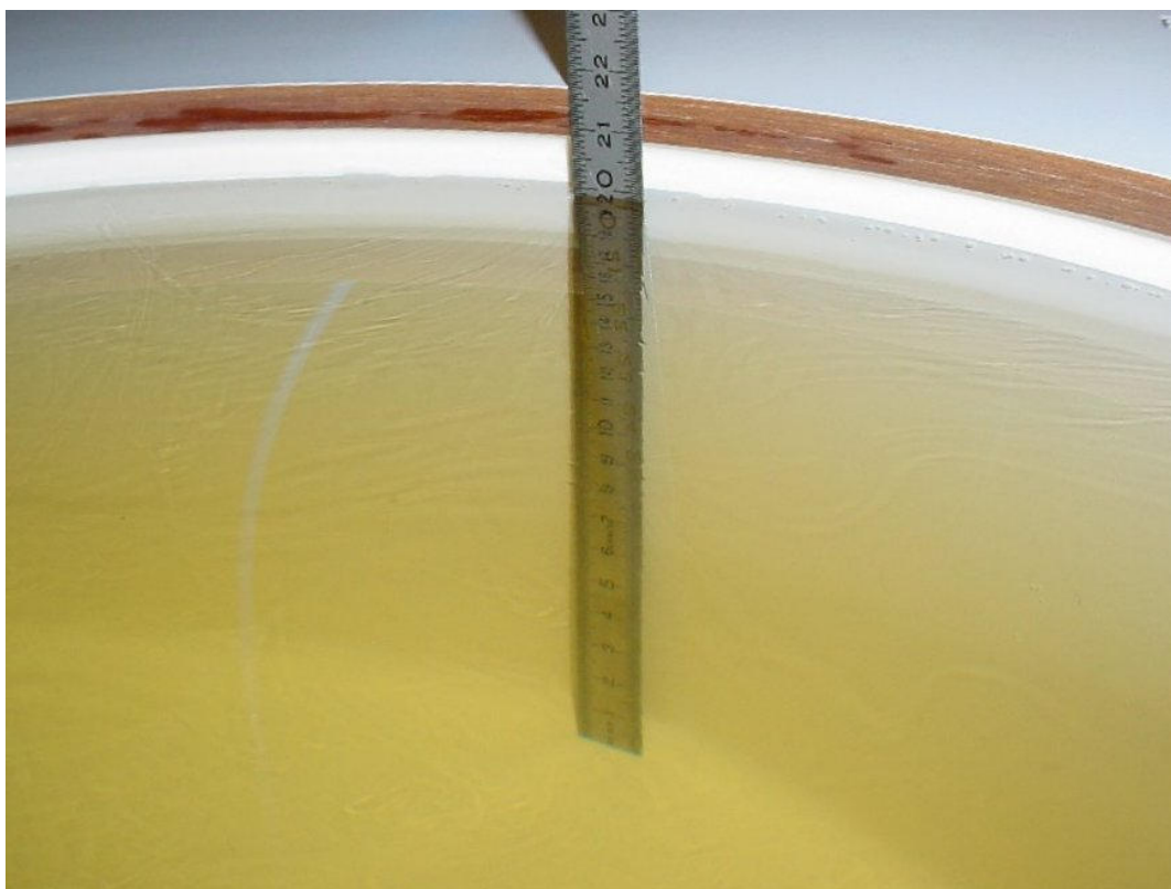
Photo 24: Liquid depth 1900 MHz head simulating liquid
