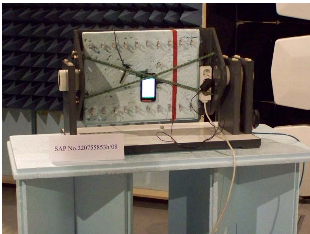
Photograph 2: Radiated field strength set-up
