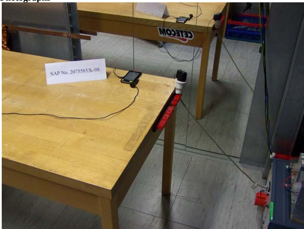
Photograph 1: Conducted emissions measurement set-up
