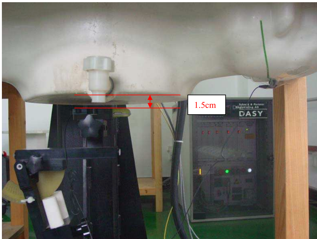
Picture B7: Body-worn Position with headset (towards ground, the distance from handset to the bottom of the Phantom is 1.5cm)
