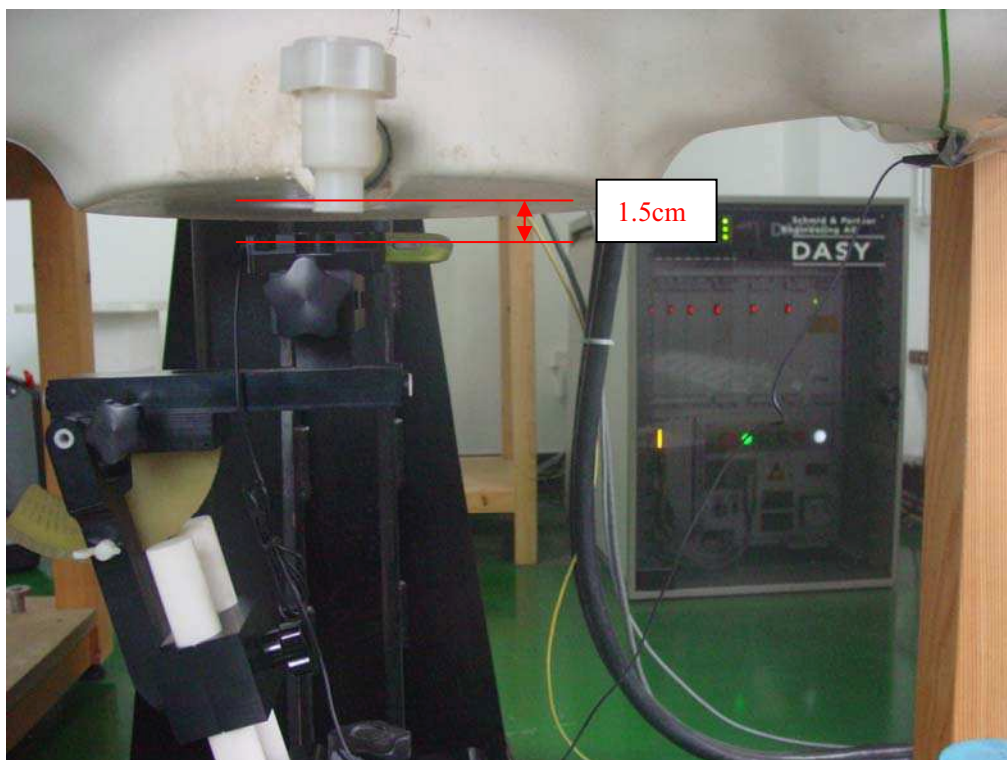
Picture B8: Body-worn Position with headset (towards phantom, the distance from handset to the bottom of the Phantom is 1.5cm)
