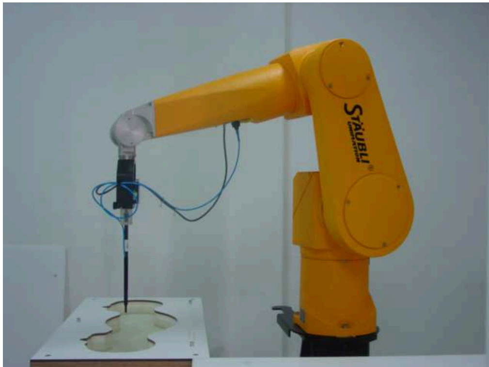
Picture B1: Specific Absorption Rate Test Layout
