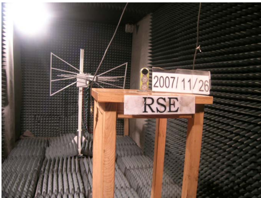
Pic2 Radiated Spurious Emission
