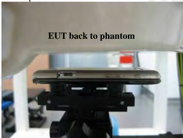
Fig.12 Body worn- EUT back to flat phantom and distance between flat phantom and mobile phone is 1.5 cm
