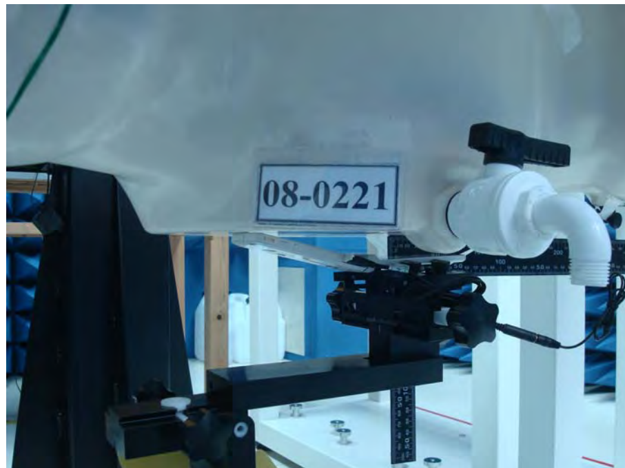
Figure 22.Body SAR Test Setup (Flat Section) _ EUT Open LCD to Phantom 15 mm separation
