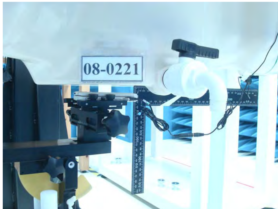
Figure 24.Body SAR Test Setup (Flat Section) _ EUT Close Top to Phantom 15 mm separation
