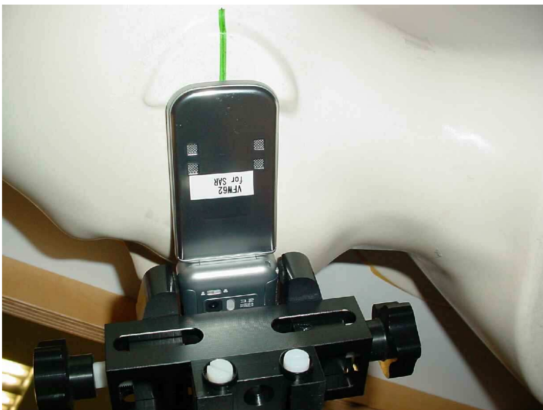
Photo 13: Test position left hand touched
