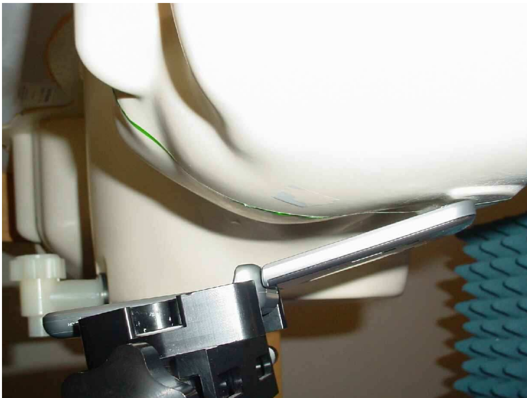
Photo 15: Test position left hand tilted 15°
