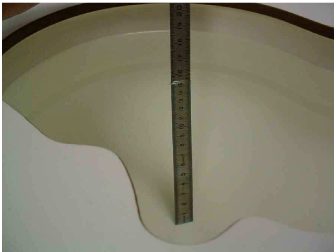
Photo 25: Liquid depth 1900 MHz body simulating liquid
