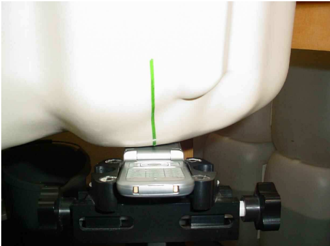
Photo 11: Test position left hand touched
