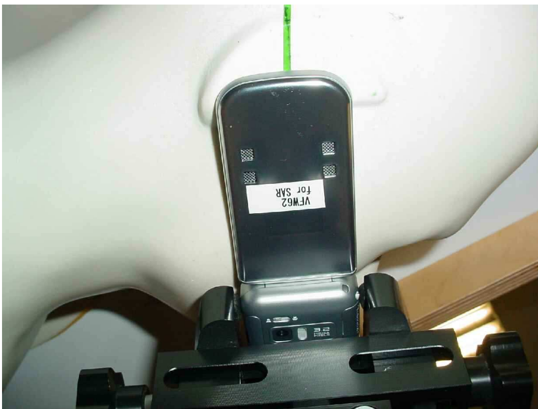
Photo 19: Test position right hand tilted 15°
