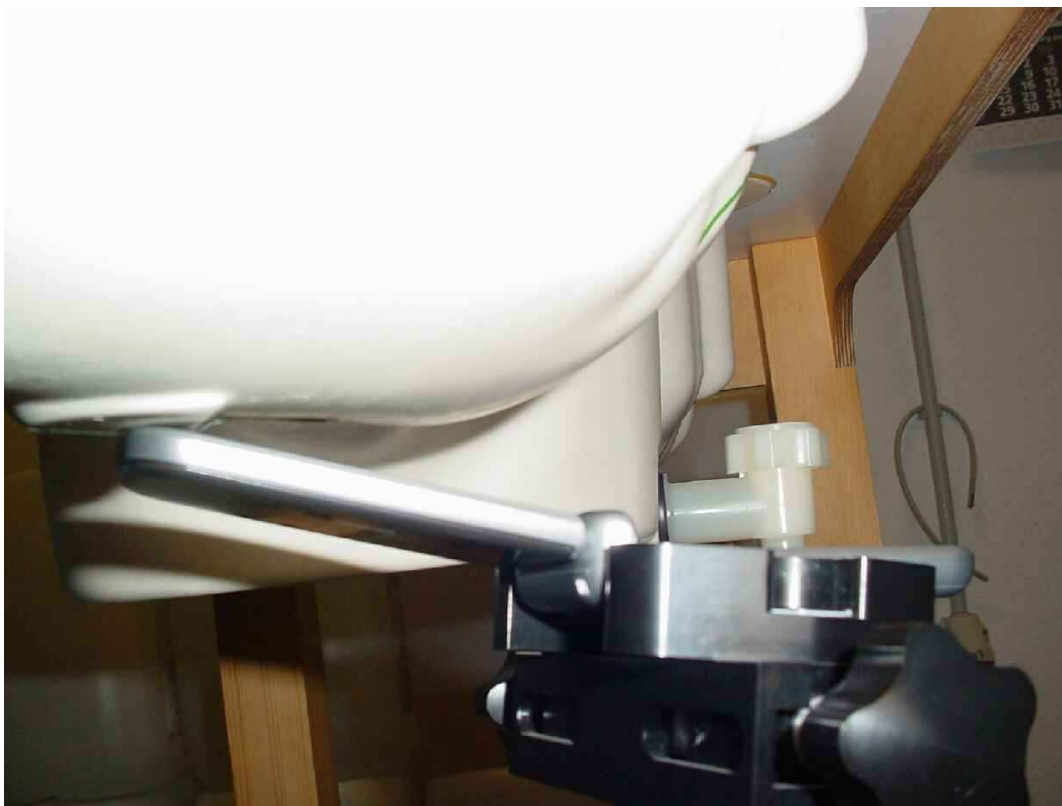
Photo 21: Test position body worn front side (distance 15 mm)
