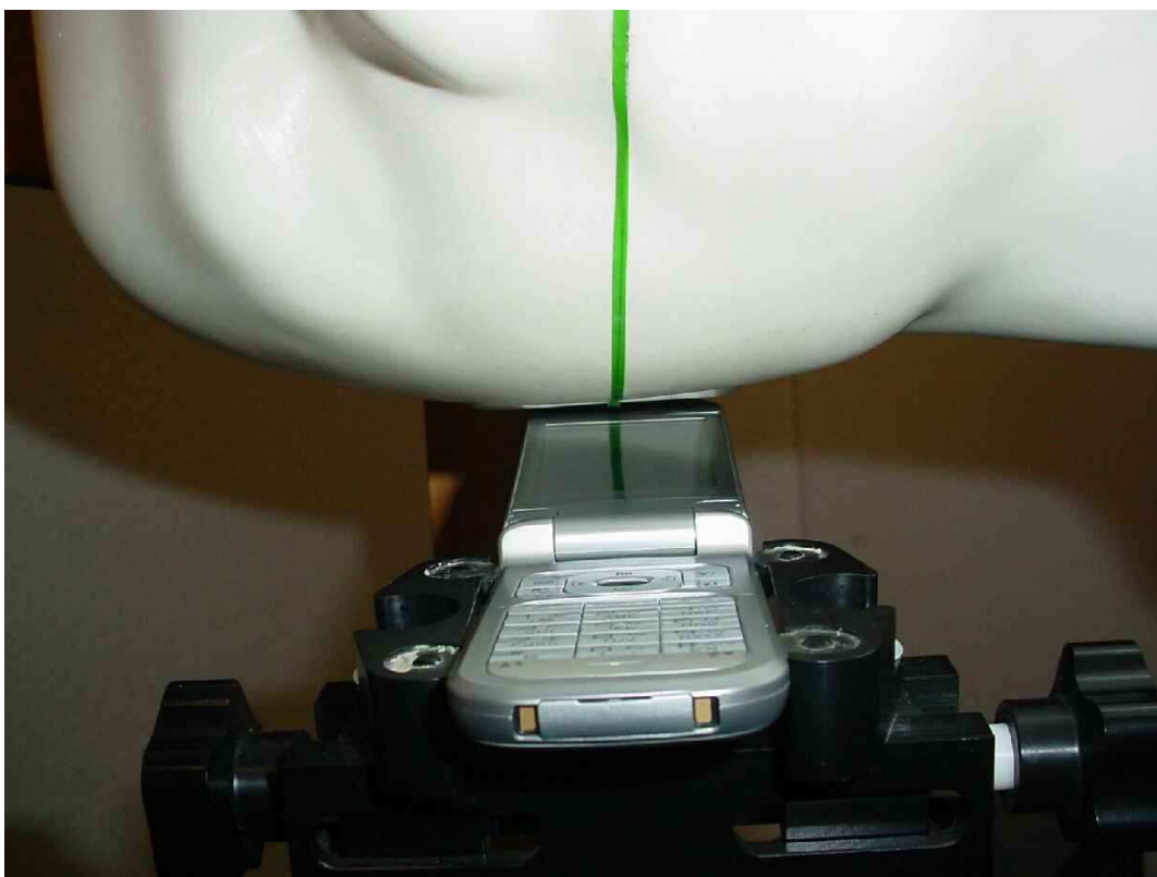
Photo 19: Test position right hand tilted 15°
