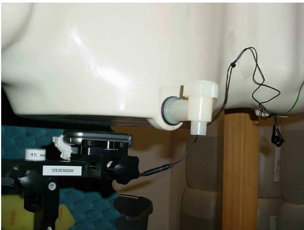
Photo 21: Test position body worn front side (distance 15 mm)
