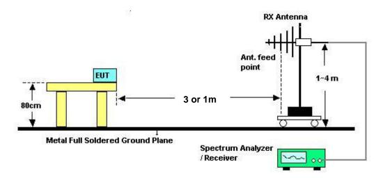
Above 10 GHz shall be extrapolated to the specified distance using an extrapolation factor of 20 dB/decade form 3m to 1m.
