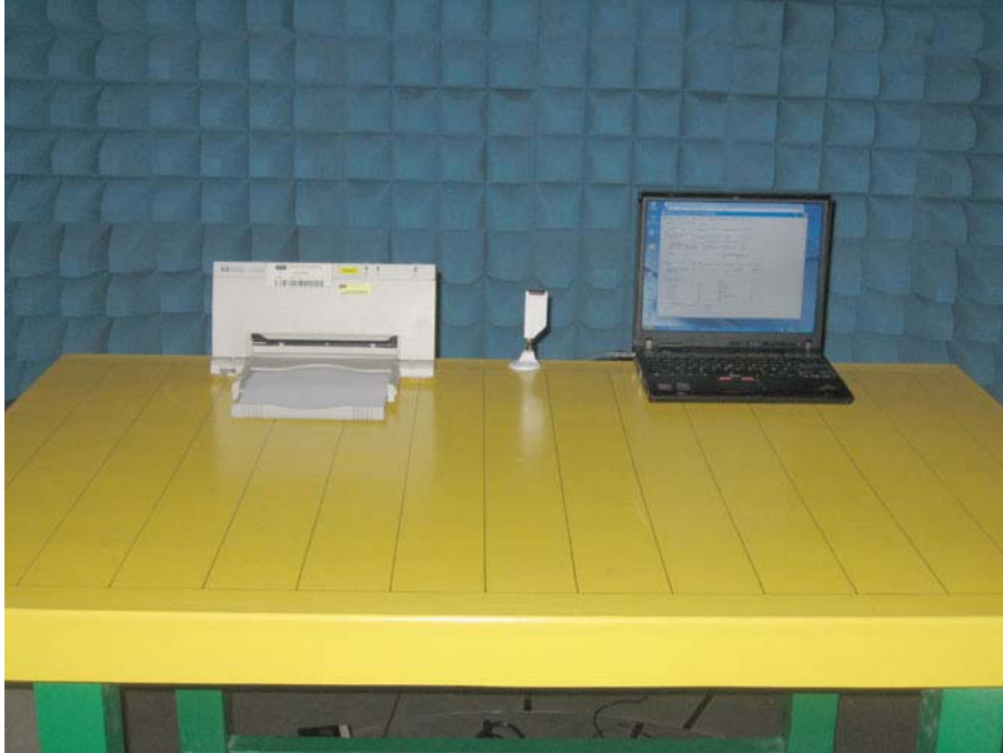
Photo 2: Radiated Emission Test Set-up
