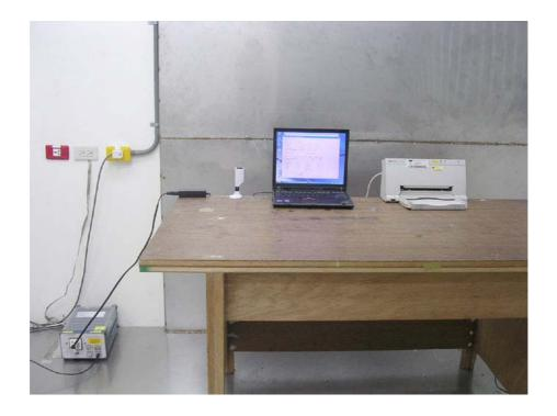
**Photo 2: Conducted Emission Test Set-up**
