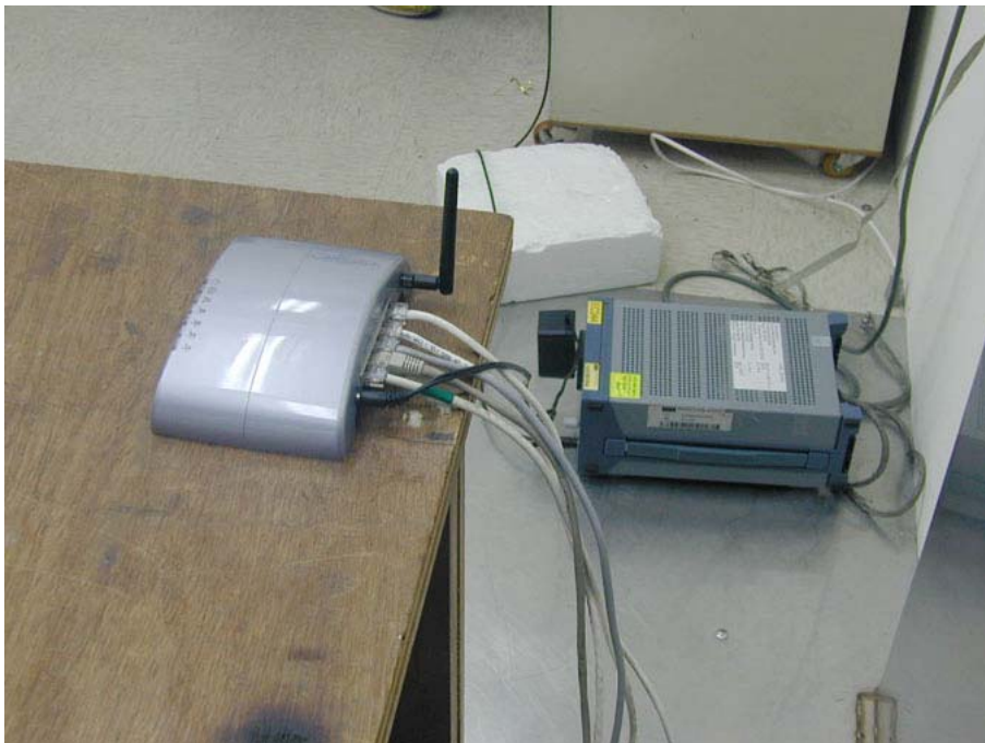
Photo 2: Conducted Emission Test Set-up
