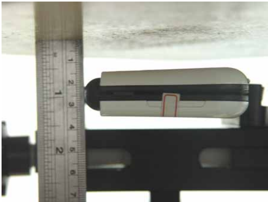
Fig. 9.8 Keypad Down with 1.5cm Gap
