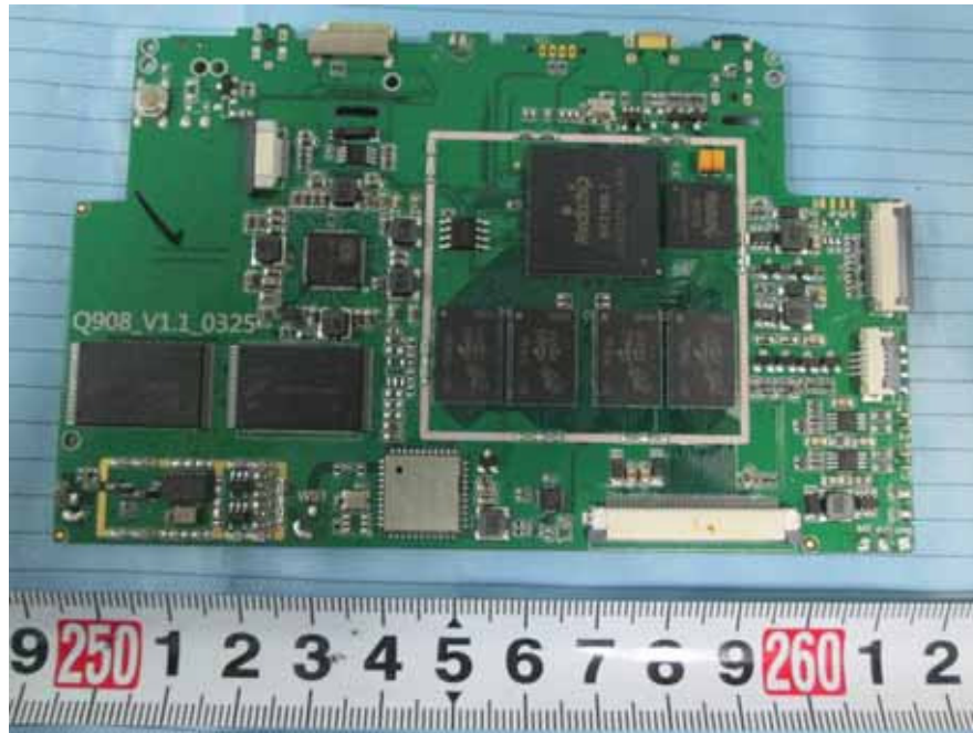
EUT – Main Board Top Shielding Off View
