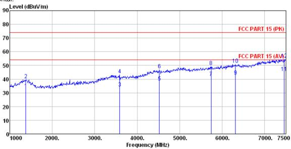
: 3m chamber : FCC PART 15 (PK) 3m BBHA9120D ANT(>1GHZ) HORIZONTAL Condition
