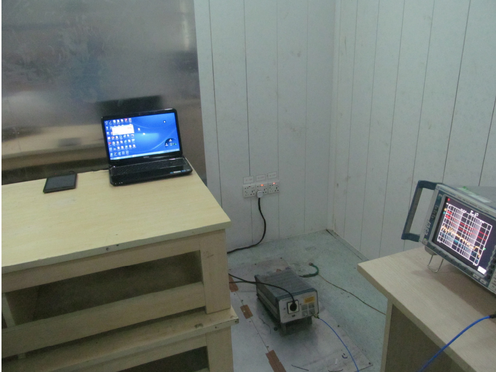
FCC RADIATED EMISSION TEST SETUP
