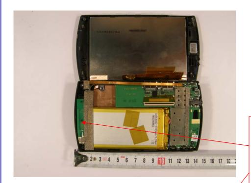
The antenna used for WiFi and Bluetooth on Archos model 7502 is a "F" antenna, directly printed on the PCB. The gain of the antenna is -3.1 dBi.
