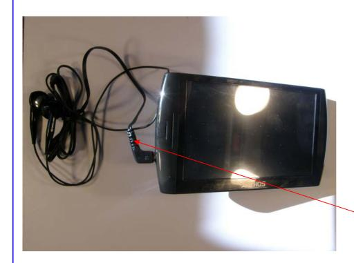
The FM receiver uses the power head set cord for antenna
