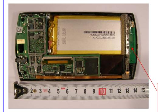
The antenna used for WiFi and Bluetooth on Archos model 7501 is a "F" antenna, directly printed on the PCB. The gain of the antenna is -3.1 dBi.
