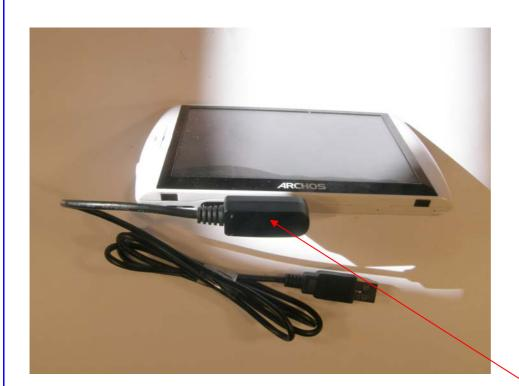
The FM band II transmitter uses the power supply cord for antenna
