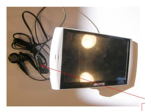
The FM receiver uses the power head set cord for antenna
