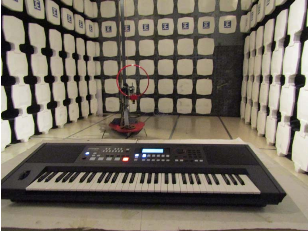
Measurement of Radiated Emission Test Set Up
