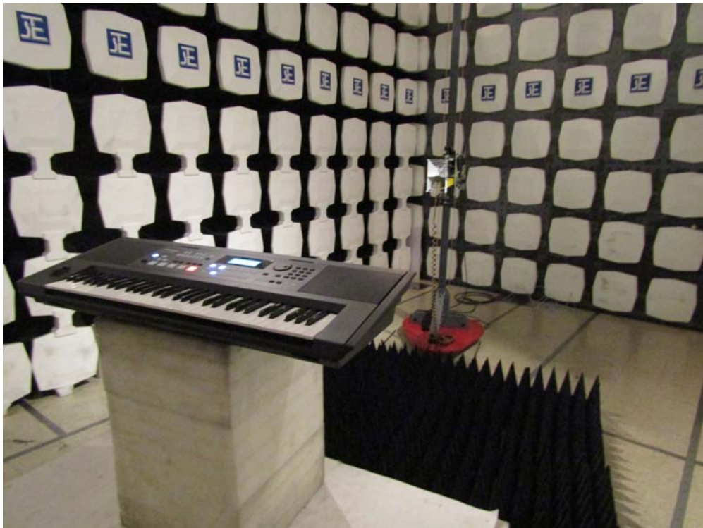
Measurement of Radiated Emission Test Set Up
