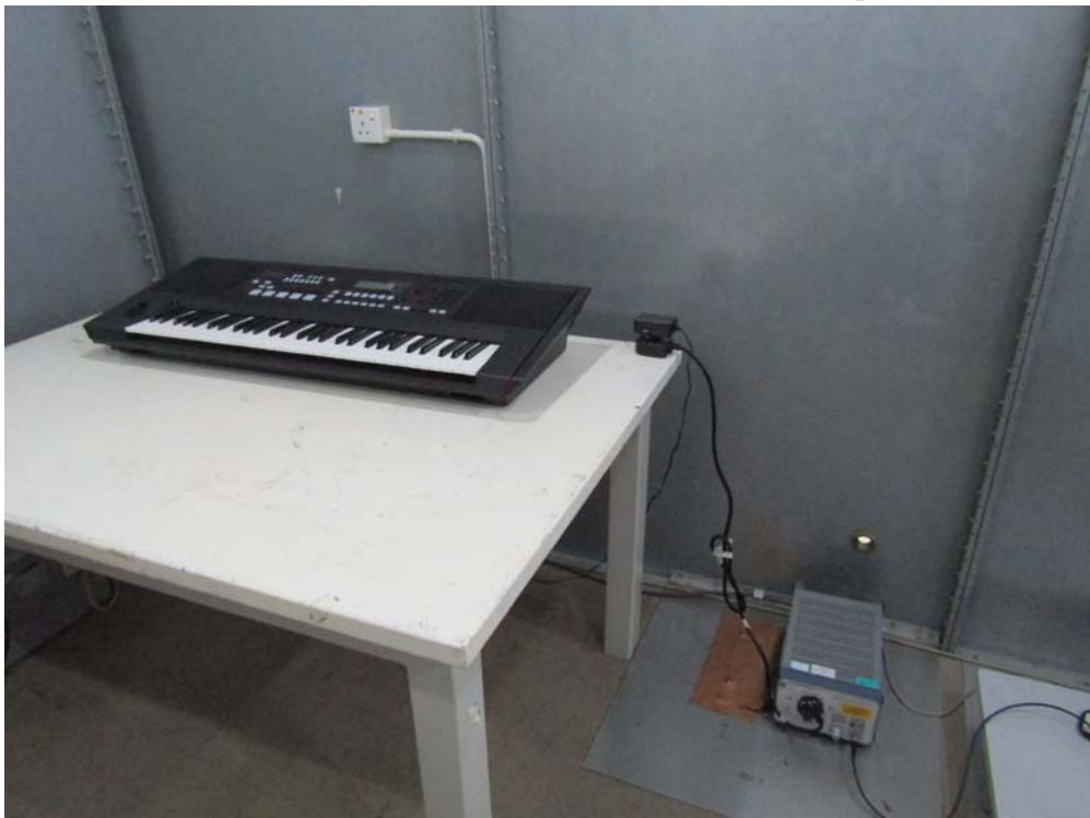
Measurement of Conducted Emission Test Set Up
