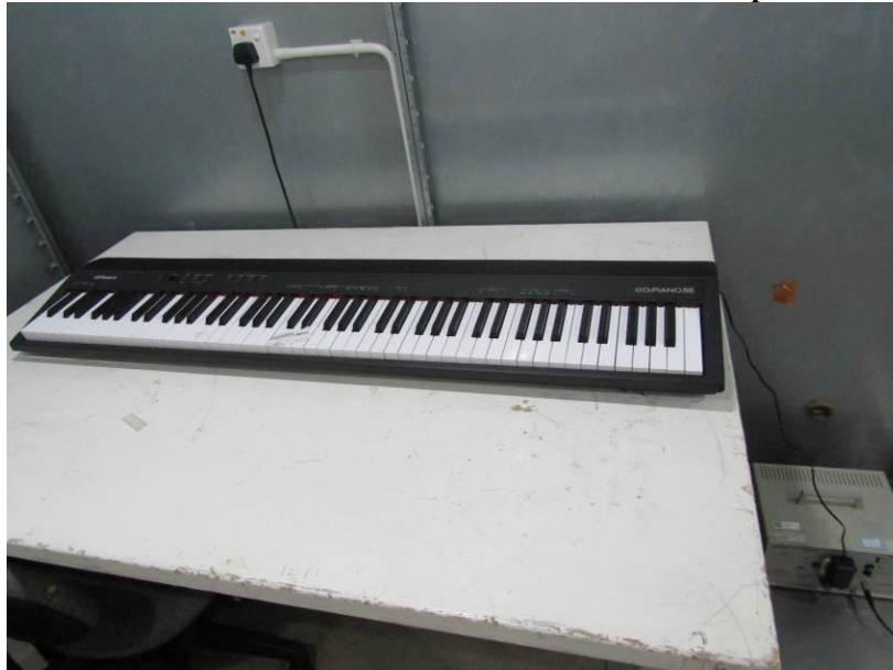
Measurement of Conducted Emission Test Set Up
